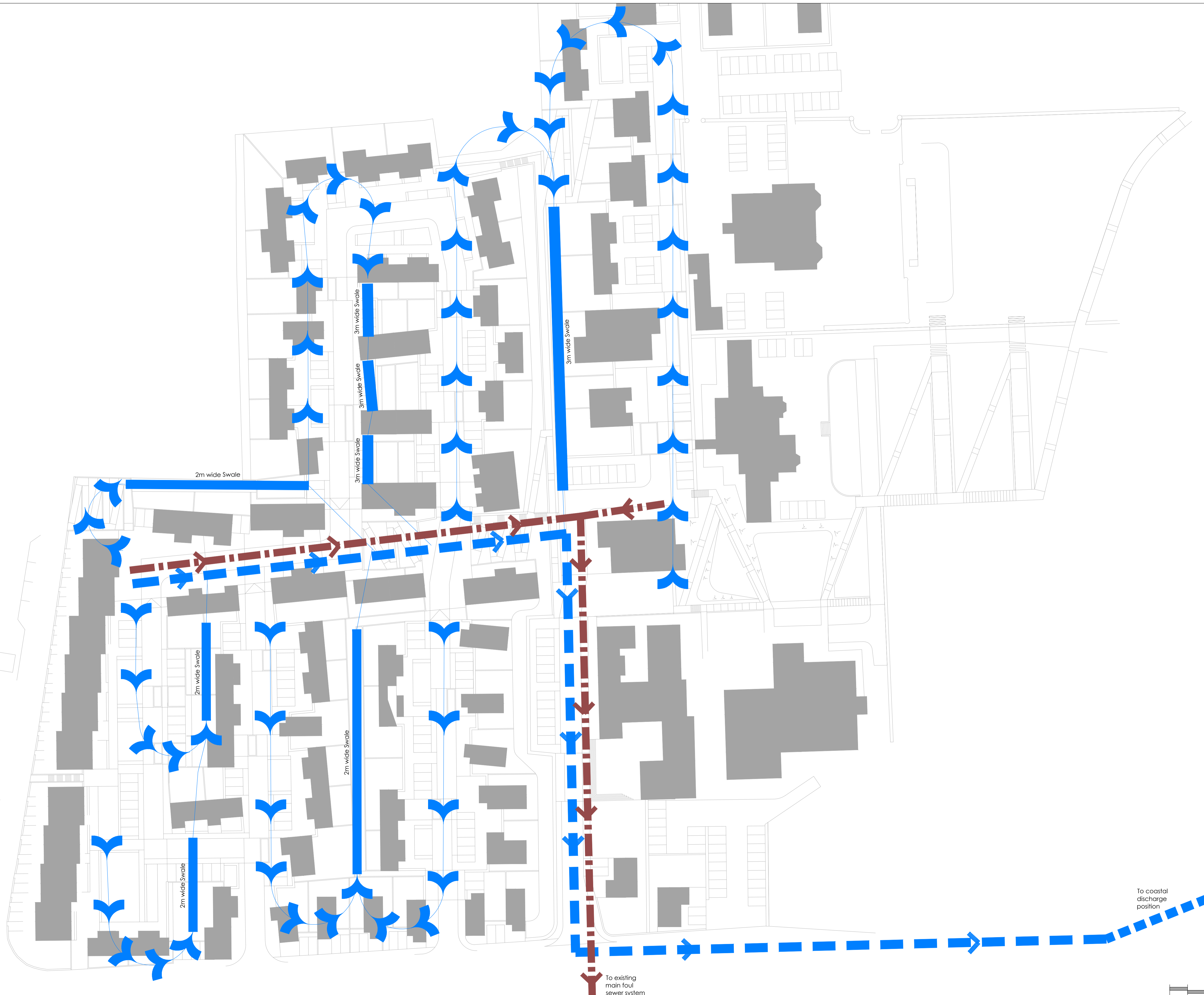
INDICATIVE DRAINAGE SCHEME SCALE 1:500
