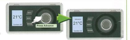
If the heater is in 'Comfort Off' mode and you want heat – press the Advance button. If the heater is in 'Comfort On' and you don't want heat, press the Advance button and it will go off until the beginning of the next 'Comfort On' period.
