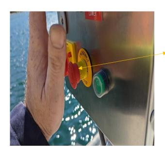
EMERGENCY STOP. Press the button to STOP. This will disable the RAISE and LOWER buttons and deactivate the electrical supply. Use in an emergency situation or on completion of lifting operations only.
