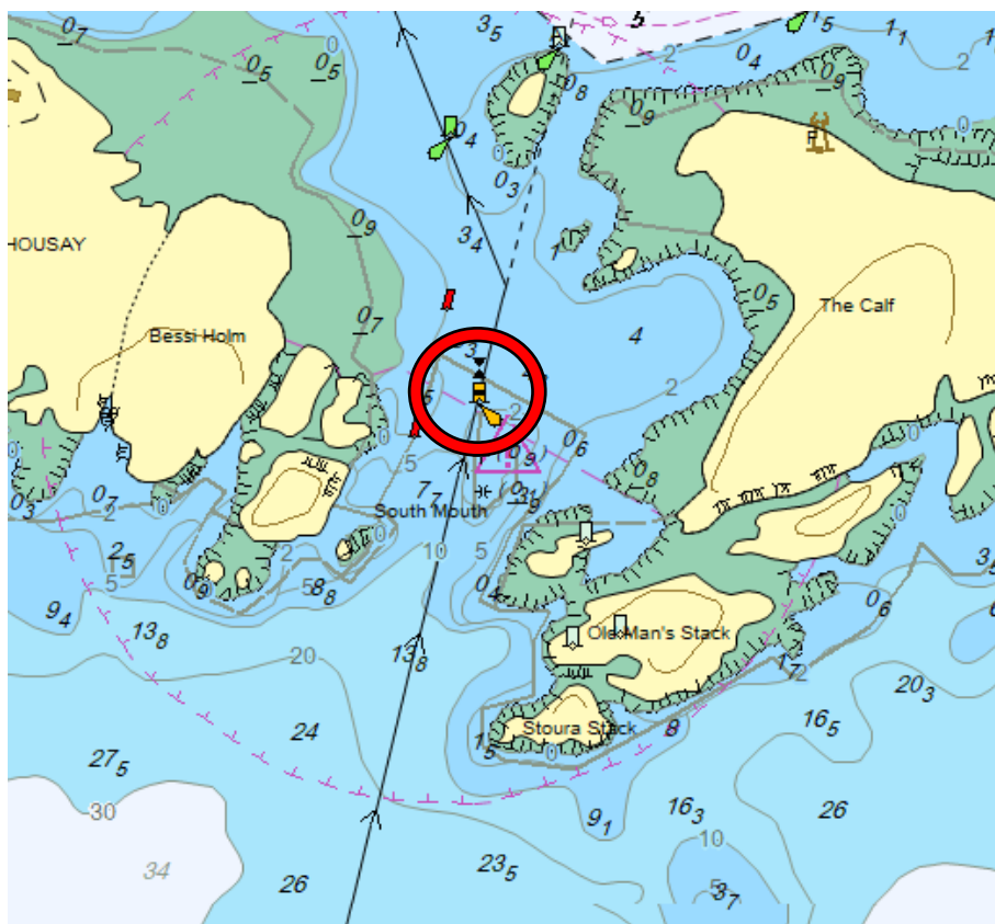
Image not to be used for navigation – unlit West Cardinal Mark shown within red circle.
